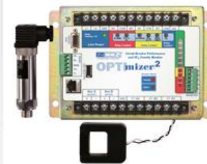
Circuit Breaker Monitor
